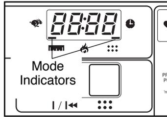
When the power is turned on, the SCAN mode will automatically be selected. One mode indicator (see the drawing above), will appear by the scan symbol, and a second mode indicator will show which mode is currently displayed.
