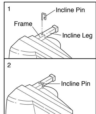
**CAUTION: Before using the treadmill, make sure that both incline pins are fully inserted at the same height. Do not use the treadmill with the incline pins removed.**
