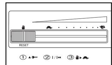
Carefully step onto the walking belt and begin walking. Change the speed of the walking belt as desired by sliding the speed control. Note: To stop
