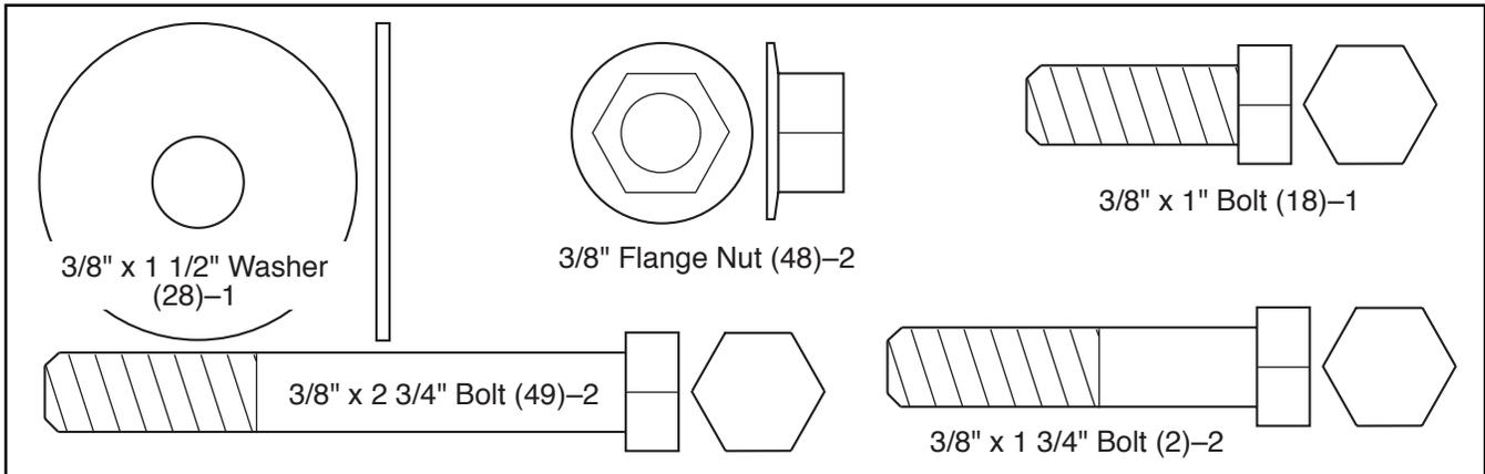
1. Raise the Upright (11) to the vertical position. Insert the 3/8" x 1" Bolt (18) and the 3/8" x 1/2" Washer (28) into the lower end of the Upright. Finger tighten the Bolt into the Frame (59).
