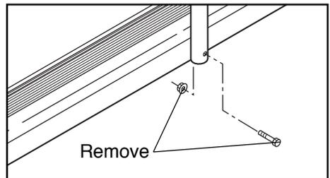
Remove the bolt from the upper end of each handrail.
