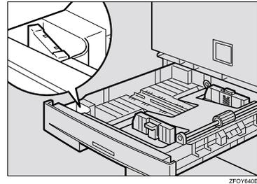
**4** While pressing the release lever, adjust the side fences.
