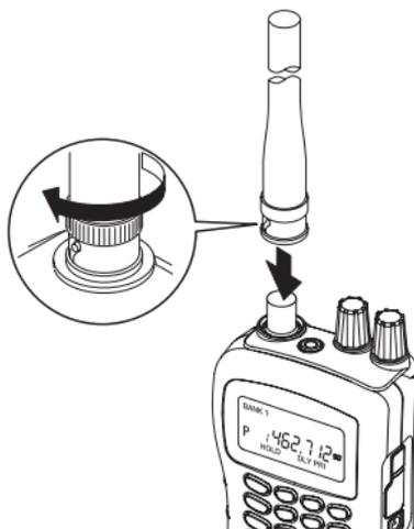
To attach the supplied flexible antenna to the connector on the top of your scanner, align the slots around the antenna's connector with the tabs on the scanner's BNC connector. Then slide the antenna's connector down over the scanner's connector and rotate the antenna connector's outer ring clockwise until it locks into place.
