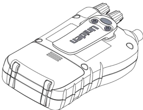
6. When **BATT** flashes and the scanner beeps every 15 seconds, replace both batteries.
