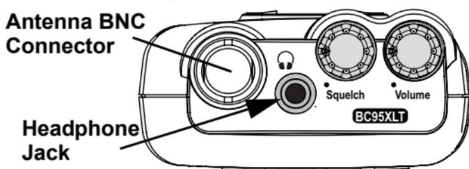
For private listening, you can plug a  $\frac{1}{8}$ -inch (3.5 mm) mini-plug earphone or mono headphones (not supplied) into the headphone jack on top of your scanner. This automatically disconnects the internal speaker.
