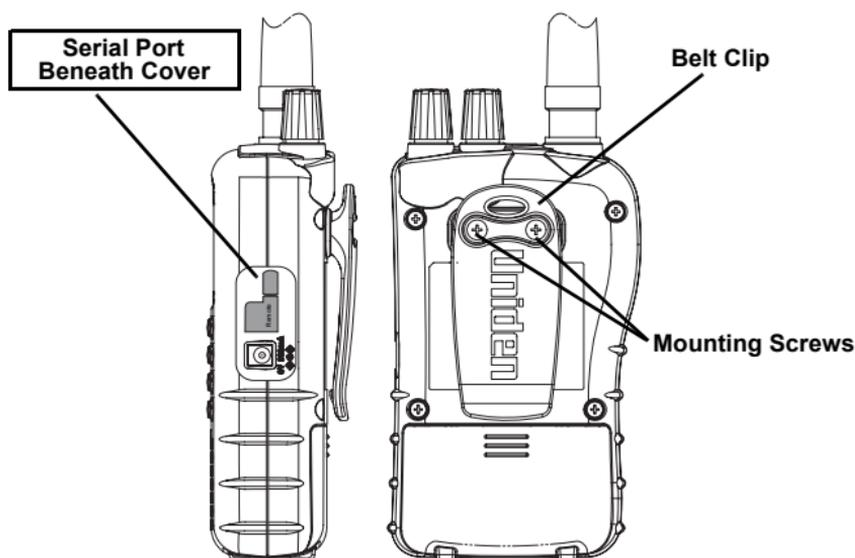
To make your scanner easier to carry when you are on the go, we provide a factory attached belt clip. Use a Phillips screwdriver to remove the mounting screws and the clip from the scanner if desired.
