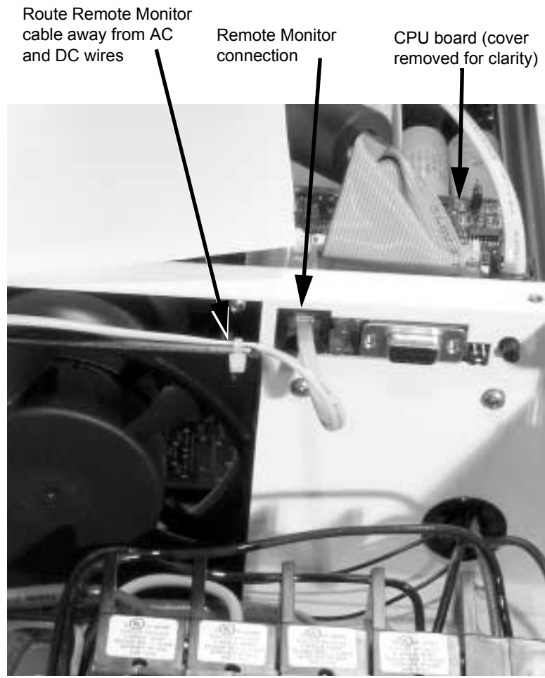
Figure 2-18 Remote Monitor connection and cable
