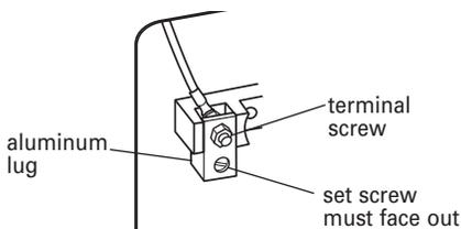
7. **IMPORTANT:** the aluminum terminal lugs must be assembled to the terminal posts with the set screws facing out as shown.
