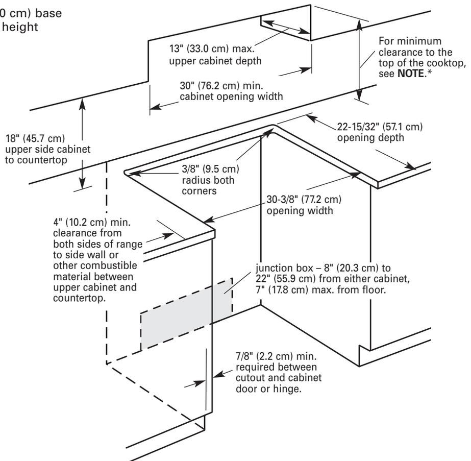
**\*NOTE:** 24" (61 cm) min. when bottom of wood or metal cabinet is protected by not less than 1/4" (6.4 mm) flame retardant millboard covered with not less than No. 28 MSG sheet steel, 0.015" (0.4 mm) stainless steel, 0.024" (0.6 mm) aluminum or 0.020" (0.5 mm) copper.
