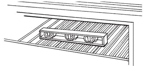
If range is not level, pull range forward until rear leveling leg is removed from the anti-tip bracket. Use 3/8" drive ratchet and channel lock pliers to adjust leveling legs up or down until range is level. Push range back into position. Check that rear leveling leg is engaged in anti-tip bracket.
