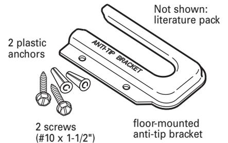
Brackets must be securely mounted to sub-floor. Thickness of flooring may require longer screws to anchor bracket to sub-floor. Longer screws are available from your local hardware store.
