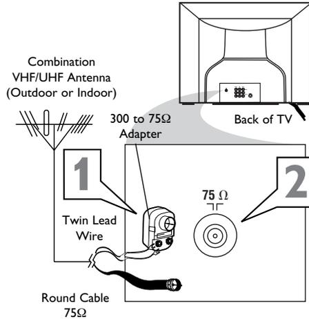
**2** Connect the Cable TV cable or Antenna cable (or 300 to 75 ohm adapter) to the 75Ω plug on the TV.
