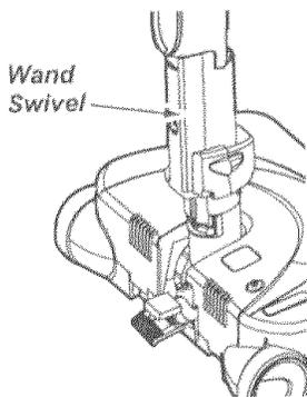
The swivel, located on the PowerMate, allows you to turn the handle to the left side to reach farther under low furniture.
