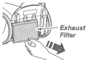
2. Pull the exhaust filter up and out from the rear of the canister.
