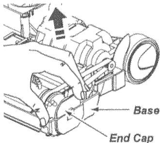
6. Check and clean end cap areas. See **AGITATOR ASSEMBLY** for picture of complete agitator assembly.
