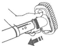
2. Slide attachments firmly on handle as needed. See **ATTACHMENT USE TABLE**.
