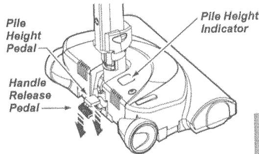
3. Lower wand from upright position by pressing on the handle release pedal.
