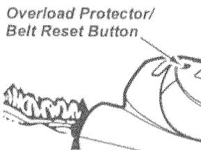
**To correct problem:** Turn off and unplug vacuum cleaner, remove obstruction, then press **BELT RESET** button. A ball point pen may be required.
