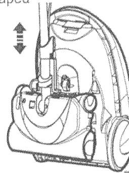
To attach the PowerMate, it must be in the flat position as shown in the illustration. Use the handle release pedal to place it in this position.
