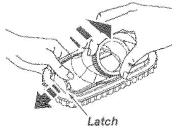
To remove, press latch and lift out.
