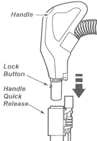
2. Insert handle into wand until lock button snaps in place. **Be sure hose is not twisted.**
