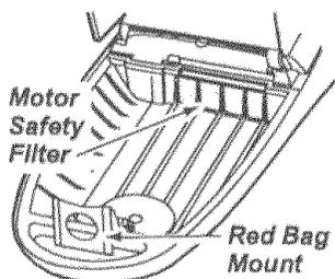
6. Check the motor safety filter and replace, if necessary.
