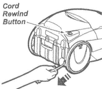
1. Pull cord out of canister to desired length. The cord will not rewind until the cord rewind button is pushed.
