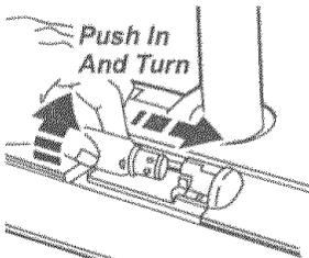
2. Push in and turn bulb counterclockwise, then pull out to remove.
