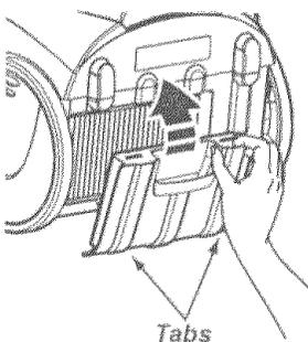
4. Replace the exhaust filter cover by placing the two tabs on the filter cover into the slots on the canister and rotate into place until it snaps closed.
