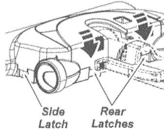
4. Rotate cover back. Press cover firmly until side and rear latches snap into place.
