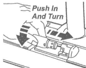
3. Push in and turn bulb clockwise, to replace. Bulb must not be higher than 15 Watts (130 Volts).
