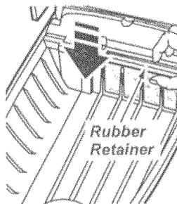
3. Replace the filter, **white side out**, facing the dust bag, by sliding it back into place under the ribs in the bag cavity. Tuck filter in so that it fits completely under the rubber retainer.
