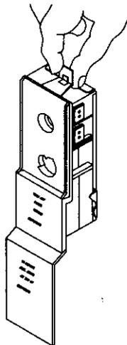
7. Disconnect the two wires on the element and unscrew the old element from the tank.
