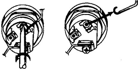
6. The buss bar is labeled 5500 W. Place the buss bar over terminals 2 and 3 with the 5500 W visible. Install the extra screw provided into terminal 3.
