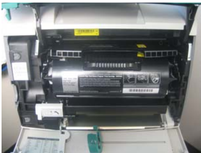
Print cartridge — 6,000 page standard — is accessible from the front of the IBM Infoprint series.
