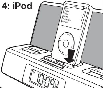
Insert iPod® into dock (iPod must not be in a "skin" or case). iPod will charge while docked. Press the iPod/play Button on the iH27 to play your iPod.
