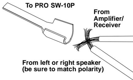
2. Position the twisted wire ends between the open barrel ends of the Speaker Pin.
