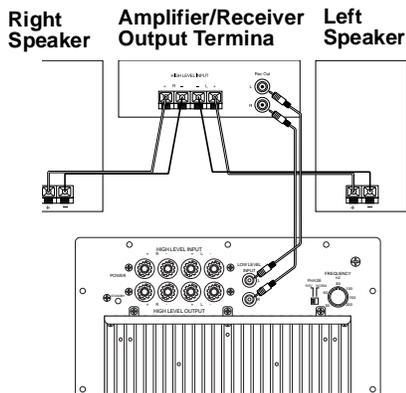
**Note:** We recommend you connect the subwoofer to an amplifier or receiver that has at least two sets of line out jacks. Connecting the subwoofer to an amplifier or receiver with only one set of line out jacks might result in no sound from the satellite speakers. If your amplifier has only one set of line out jacks, follow the instructions under "Connecting to Speaker Terminals" instead.
