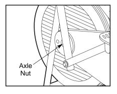
straight and retighten the axle nuts.
