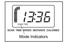
a second mode indicator will show which mode is currently displayed. Note: If a different mode is selected, you can select the scan mode again by repeatedly pressing the mode button. Time, speed, distance, or calories mode—To select one of these modes for continuous display, press the mode button
