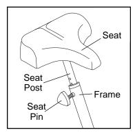
pin counterclockwise to remove it. Next, align a different hole in the seat post with the hole in the frame, and insert the seat pin into the frame and the seat post. Make sure to insert the seat pin into the seat post; do not insert the seat pin under the seat post. Tighten the seat pin into the frame.
