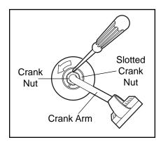
Place the end of a standard screwdriver in one of the slots in the slotted crank nut. Lightly tap the screwdriver with a hammer to turn the slotted crank nut counterclockwise until the arms are no longer loose. **Do not overtighten the slotted crank nut.** When the slotted crank nut is properly tightened, retighten the crank nut.
