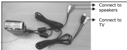
Figure 2-10: Connecting your camera to the TV
