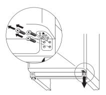
2. Remove the door fitting from the door bearing (1, 2). Move the bearing pivot from the right to the left hand hole (3). Place the door fitting supplied on the bearing pivot (4, 5).
