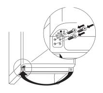
7. Move the door handle from the left to the right and cover the remaining holes with the hole cover pins attached.
