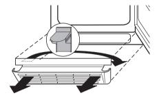
1. With the door closed, remove the cross-head screws from the lower door bearing and remove the door bearing downwards.
