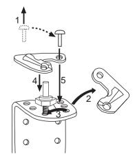
3. Remove the door fitting on the lower right (1) and reposition the door bearing cover from the lower left to the right of the door (2), place the door fitting supplied in the lower left of the door (3). Carefully remove the door to the front and place on one side.
