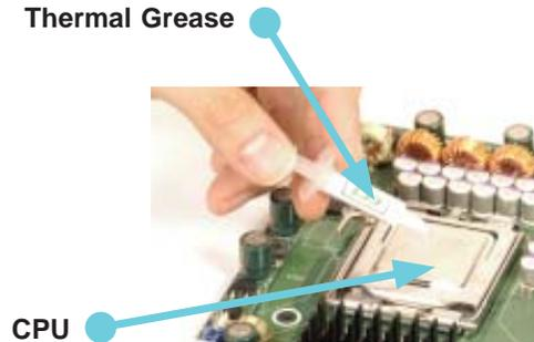
3. Apply the proper amount of thermal grease on the CPU. If your heatsink came with a thermal pad, please ignore this step.
