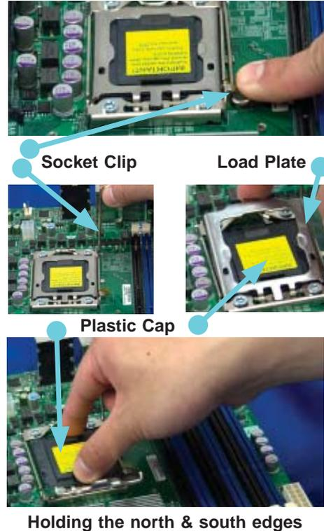
1. After removing the plastic cap, use your thumb and the index finger to hold the CPU at the north and south center edges.
