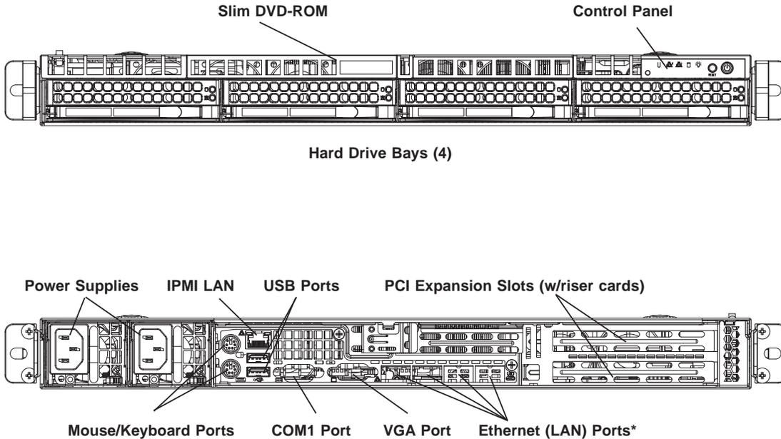
\*The 6016T-6RF+ has two 1 Gb Ethernet ports while the 6016T-6RFT+ has two 1 Gb and two 10 Gb ports.
