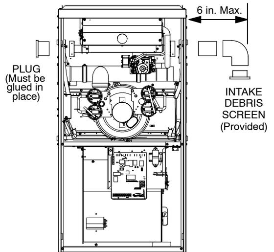
**NOTE** - Debris screen and elbow may be rotated, so that screen may be positioned to face forward, backward or downward.
