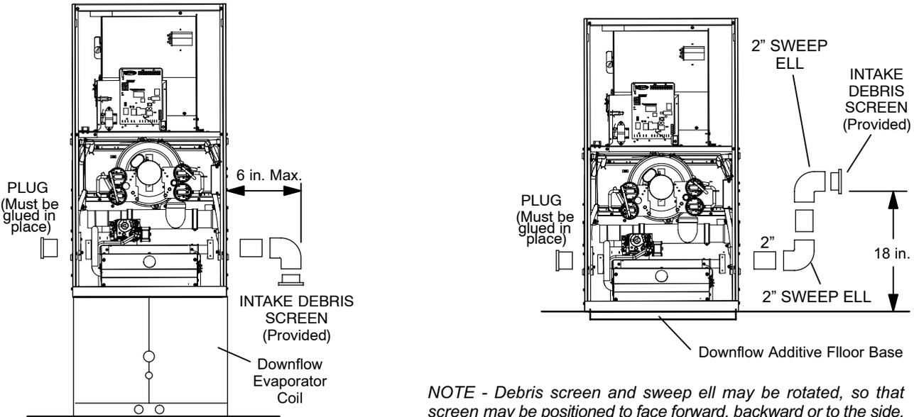
*NOTE - Debris screen and sweep ell may be rotated, so that screen may be positioned to face forward, backward or to the side.*
