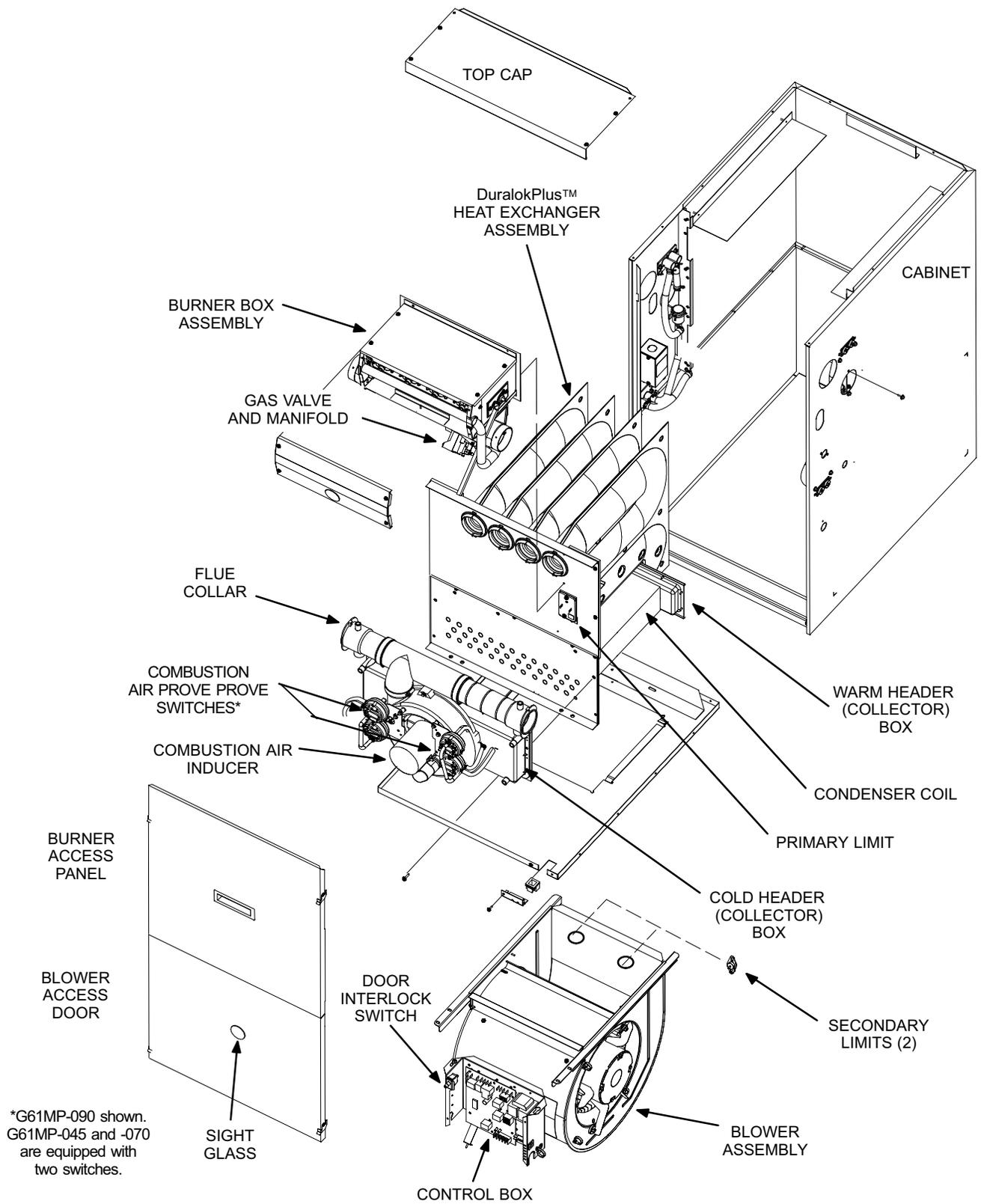
\*G61MP-090 shown. G61MP-045 and -070 are equipped with two switches.
