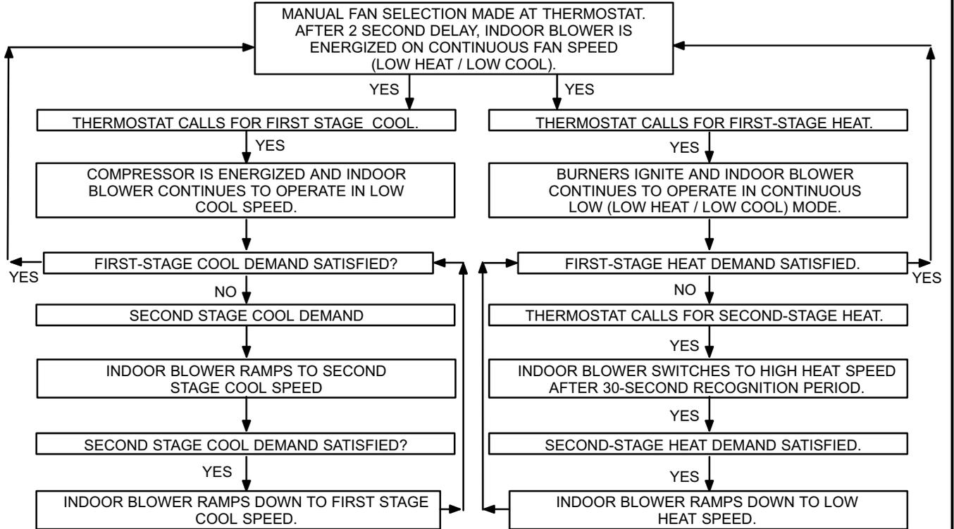
*NOTE - Continuous low speed fan and cooling low speed are equal to the low heat fan speed.*
