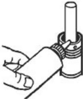
*Failure to lubricate the piston properly with throat seal oil can cause premature wear and damage to piston and packings.*
