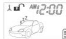
**Note:** The LCD transmitter will show Z's on the display to indicate in the Valet mode.
