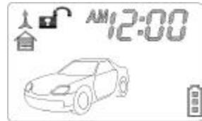
**TAMPER DISARMING:** If the alarm was triggered in your absence, when disarming the system, the siren will chirp 4 times and the parking lights will flash 3 times, indicating an intrusion to the security system while you were away from the vehicle.
