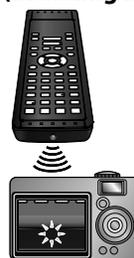
Point a digital camera towards the remote control. Push any button on the remote control and look through the digital camera. If the infrared light appears through the camera, the remote control is working.
