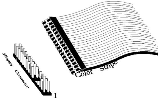
The motherboard supports up to two 720 KB, 1.44 MB, or 2.88 MB 3½" drives and 360 KB and 1.2 MB 5¼" drives. The connecting cable is a 34-pin ribbon connector with two 34-pin edge connectors for attaching the floppy disk drives. There is a small twist in the cable between the floppy connectors. The last (end) connector should be connected to floppy drive A:.
