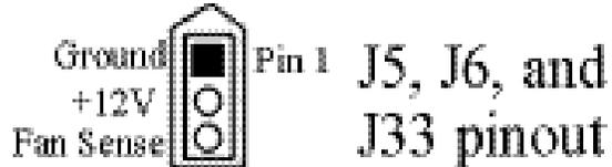
All Pentium II CPUs are shipped with a *heat sink and a CPU fan*. The connector from the CPU fan usually has three leads (has red, yellow, and black leads). *Connect the Red lead to Pin 2 (+12V). Make sure that you use fans that have 3 leads.* The 3<sup>rd</sup> (yellow) lead should provide a tachometer output to permit the fan speed to be monitored by the onboard server management hardware. If you must use fans with only 2 leads, connect the red lead to Pin 2.
