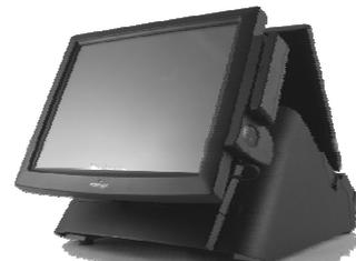
the DC power to the 2<sup>nd</sup> display, it required a qualified technician to set the power supply in XP main unit through the VGA connector according to Posiflex technical information. **Do not connect other monitor to this port before the power in this port is disabled.**
