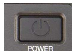
This power switch turns the system on when pushed only. This switch turns the system off when pushed again during power on status. However, if the system hangs due to any reason such as software resource conflict, a simple push on the switch in 10 sec may turn off the power.
