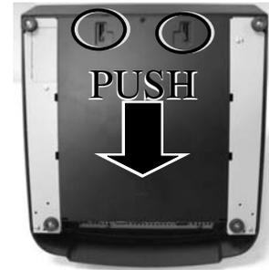
Please take it out and place it in the battery compartment at centre lower part of the bottom area as arrowed in the picture at bottom centre. Passing the cable through the groove and connect the cable to its connector in the main connection area which shown in the picture at bottom centre. Assemble the bracket after plug the connector and cover the bottom plate.
