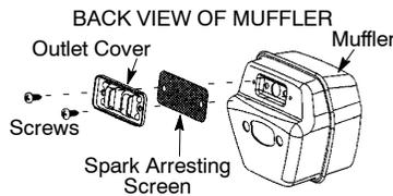
6. Clean the spark arresting screen with a wire brush. Replace screen if any wires are broken or screen is blocked after cleaning.
