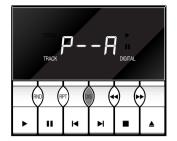
Load a disc and press OPEN. Wait until the display shows the disc time then the number of tracks. Press and hold DIS (DISPLAY) for one second. Holding for longer will enter programme mode B. To start again press **OPEN**.
