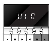
User Options. To customise the operation of the IKEMI and GENKI go to the User Options mode. Switch the power on while holding the **OPEN** button for twelve seconds. **OPEN** selects the Option, **STOP** changes its value. See the following table for the options. To exit press and hold **OPEN** for five seconds.
