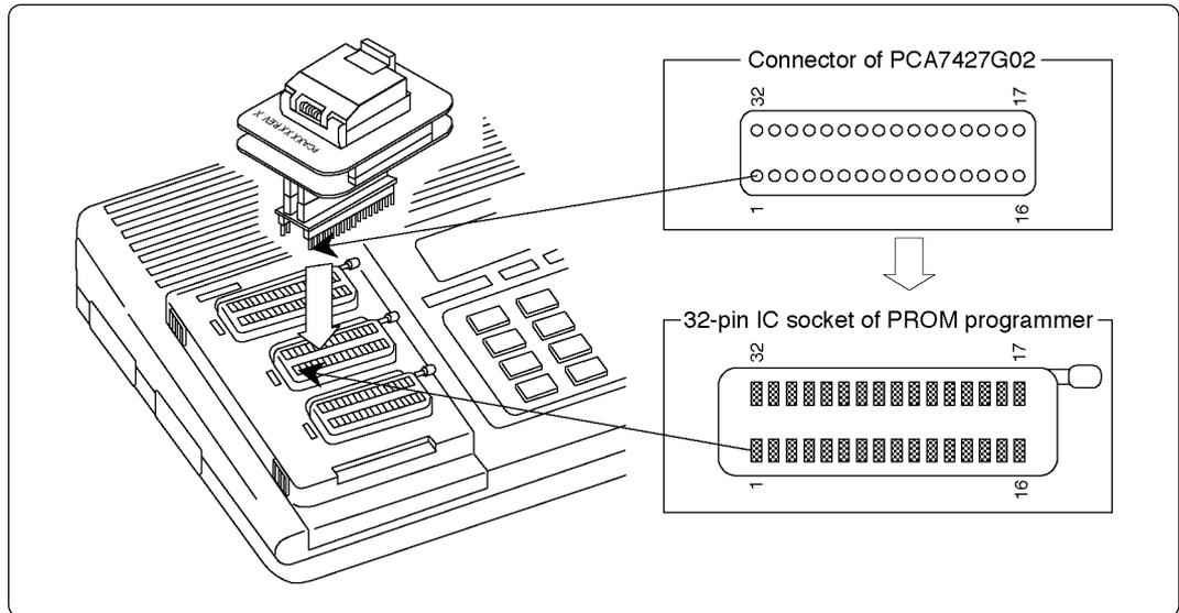
Figure 4.1 Attaching the adapter to a PROM programmer
