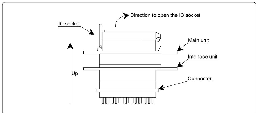
Figure 4.4 Holding the adapter in a horizontal position
