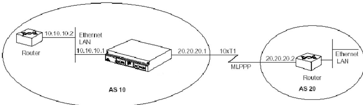
Configuring EBGP between two different autonomous systems.
