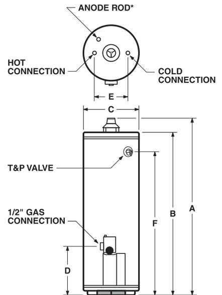
\*Location for optional top-mounted T&P Valve, if ordered from factory. To order, add "G" to model number (GPX 40 YXRTG).
