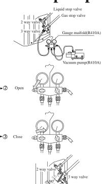
If it does not stop gas leakage, discharge whole refrigerants from the service port. After flaring work again and vacuumize, fill up prescribed refrigerant from the gas cylinder.
