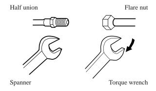
Forced fastening without careful centering may damage the threads and cause a leakage of gas.
