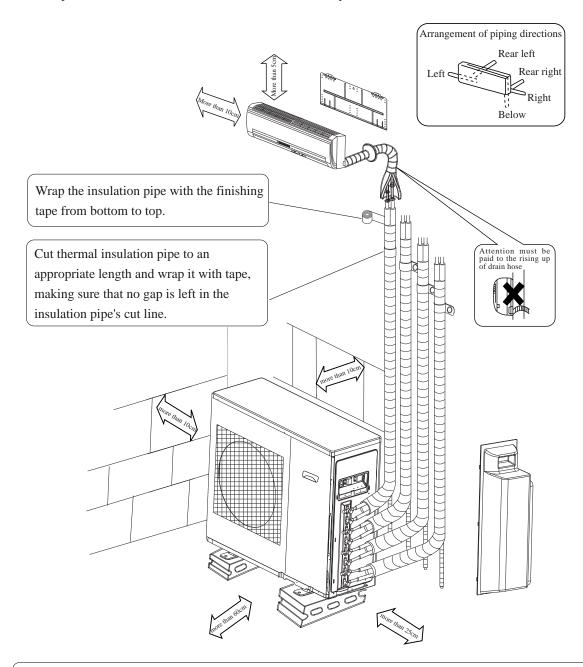
If there is the danger of the unit falling or overturning, fix the unit with foundation bolts, or with wire or other means.
