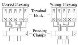
• Crimp connection method for wires without terminals
