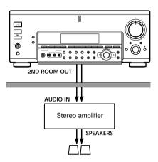
You can select the analog audio signals for output to a stereo amplifier in another room. For details on the connection, see page 13.
