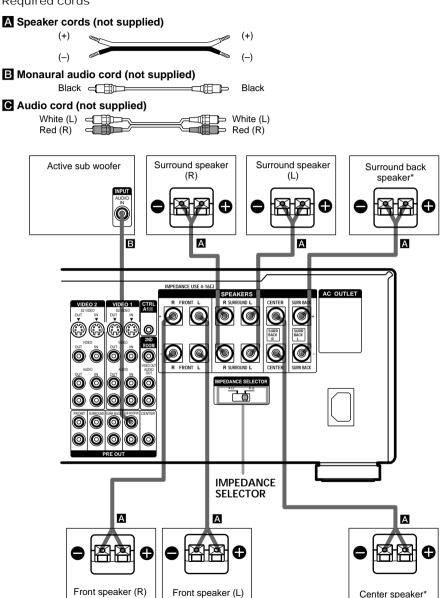
You can use the connected center and surround back speakers as surround back right and left speakers. (See "Selecting the 7.1 channel mode" on page 28.) Make sure to connect correctly as indicated on the rear panel.
