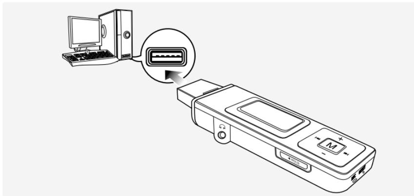
Remove the USB Cover then connect the USB Connection Plug to the USB port (
