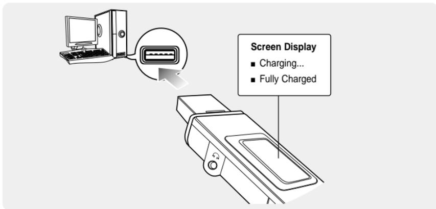
**Remove the USB Cover and then connect the USB Connection Plug to the USB port ( ) on your PC.**
