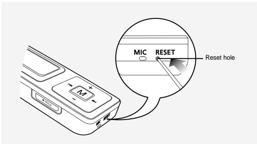
**Press the Reset hole at the bottom of the product with a pointed object such as a safety clip.**
