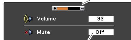
Press the MUTE button to set the Mute function **On** or **Off**. The dialog box disappears after 4 seconds.
