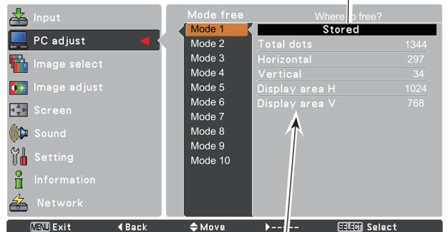
Values of **Total dots**, **Horizontal**, **Vertical**, **Display area H**, and **Display area V**.
