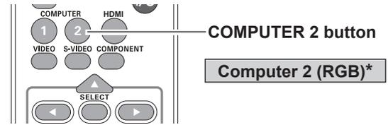
\*COMPUTER 2 can not be selected when using the COMPUTER IN 2/ MONITOR OUT terminal as MONITOR OUT output.
