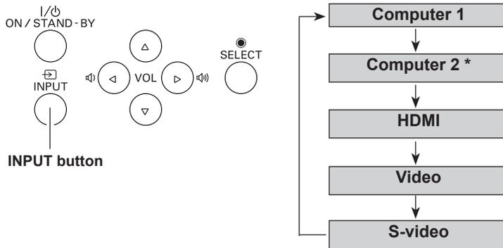
\*COMPUTER 2 can not be selected when using the COMPUTER IN 2/ MONITOR OUT terminal as MONITOR OUT output.
