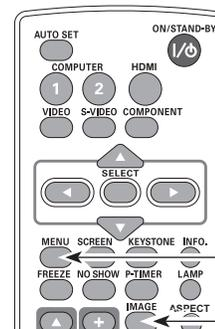
While pressing the MENU button, press the IMAGE button more than five seconds to switch between the codes.
