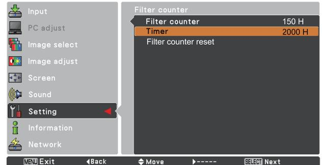
Press the SELECT button to select **Timer**, and then use the Point **▲▼** buttons to set the timer. Select from (**Off/ 2000H/ 3000H/ 4000H**) depending on the use environment.
