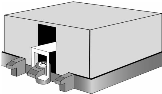
2. After tightening screws secure metal clip to plastic retention bracket center tab. Repeat for the other side of heatsink.
