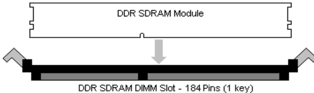
Once the memory modules are firmly seated in the slot, two latches on either side will close and secure the module into the slot. Sometimes you may need to close the latches yourself.
