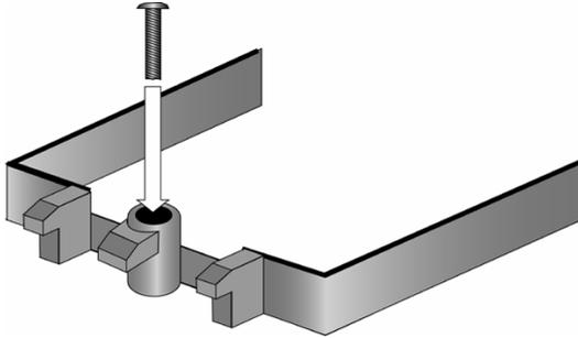
1. After placing backplate and interface material under motherboard place heatsink retention frame on top of motherboard. Align plastic retention bracket screw holes with CPU backplate standoffs. Tighten screws to secure plastic retention bracket. Repeat for the other side. **DO NOT OVER TIGHTEN.**
