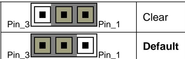
You can reset the CMOS settings by using this jumper if you have forgotten your system/setup password or need to clear system BIOS setting.
