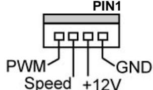
Use these connectors to connect processor cooling fans to your motherboard.
