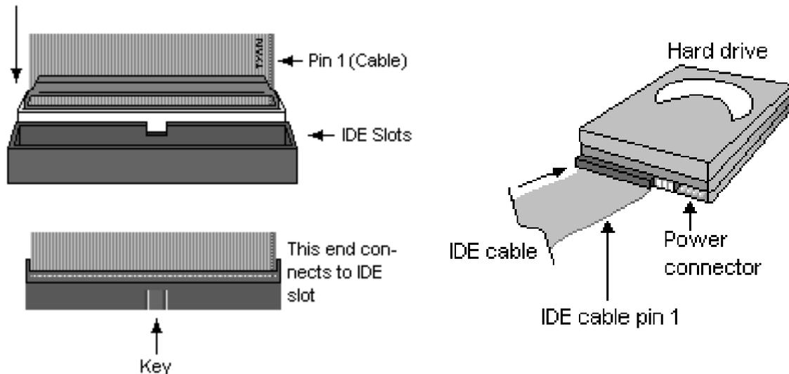
Simply plug in the BLUE END of the IDE cable into the motherboard IDE connector, and the other end into the drive. Each standard IDE cable has three connectors, two of which are closer together. The BLUE connector that is furthest away from the other two is the end that connects to the motherboard. The other two connectors are used to connect to drives.
