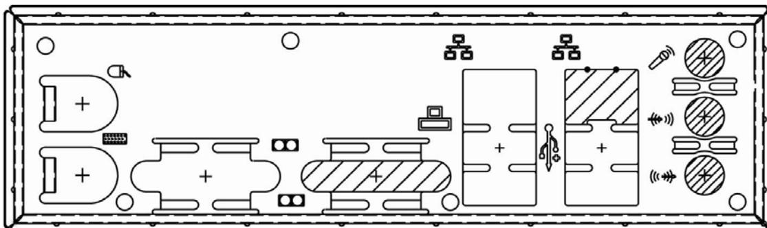
The VGA port, GbE LAN2(BCM5705) port and Audio ports are covered with soft metal which can be disassembled easily by hand.
