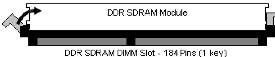
To remove the memory module, simply push the latches outwards until the memory module pops up. Then remove the module.
