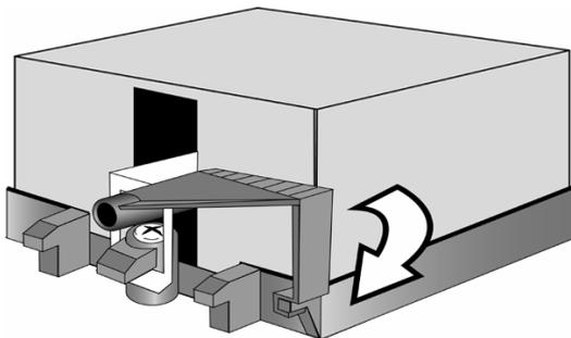
3. After securing metal clip to plastic retention bracket center tab, push down on plastic clip to lock plastic clip to side tab.
