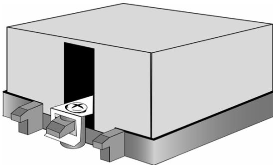
3. Tighten screw through metal clip. Repeat on the other side. **DO NOT OVER TIGHTEN.**
