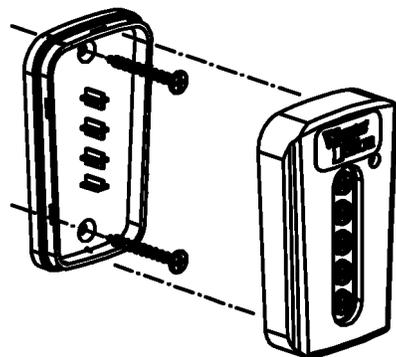
Snap open the Wireless Keyless Entry case with a coin. Secure keyless entry base into wood wall framing using the two screws provided. Snap the front case half with the base. Remove paper backing from instruction label and apply to a clean surface inside garage.
