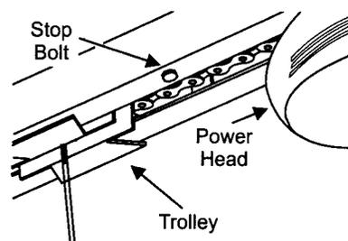
To confirm final OPEN travel adjustment, activate the opener to bring door to fully open position. The opener light should **not** be flashing.
