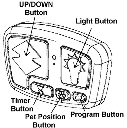
To set a custom pet position, start with the door in the closed position.
