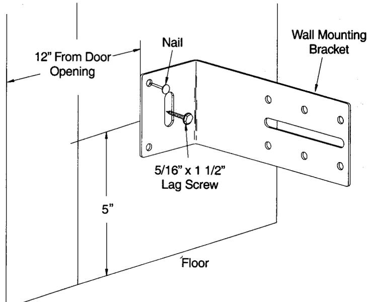
The brackets may be temporarily mounted to the jamb with a 1" flat head nail (provided), permanently mount the wall mounting bracket to both door jambs. In some installations it may be necessary to attach wooden spacers to the wall to achieve the required clearance. Expansion bolts (not included) may be required to attach brackets to walls constructed of materials other than wood or gypsum.
