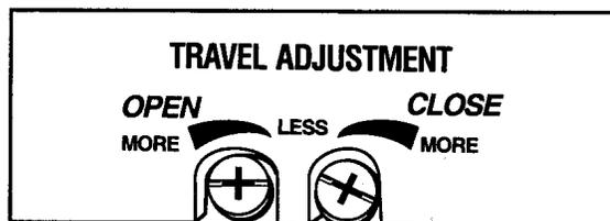
To determine the door's "natural" fully open, resting position, disconnect door from opener using the Emergency Release Disconnect (see page 26, HOW TO OPERATE YOUR DOOR MANUALLY) and manually raise door to its "natural" fully open, resting position. Use this location for your open limit setting. To determine if door needs adjustment, activate the opener to bring door to fully open position.
