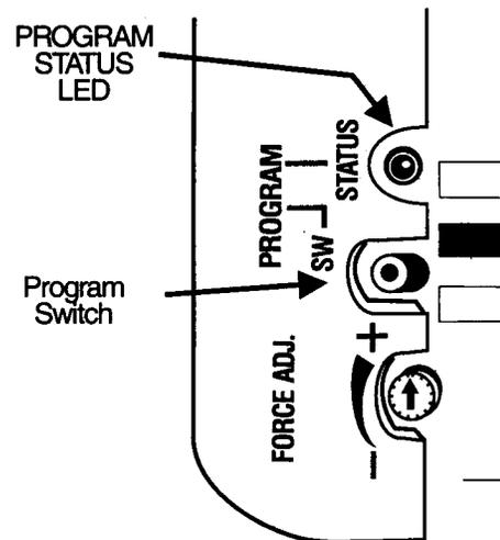
At this point you will be able to activate the opener. It will open, but will not close the door. Before unit will close door the beam sensors must be aligned and programmed (next step).
