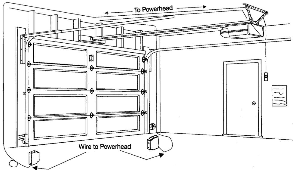
**Note:** *If wires must be lengthened or spliced into pre-wired installation, use wire nuts or a suitable connector.*
