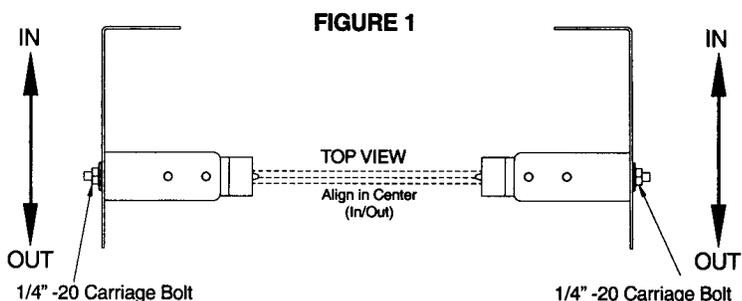
Once the alignment light comes on, tighten all bolts and mounting screws.
