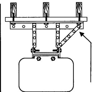
For finished ceilings, or if structural beams are out of position for mounting, use a third mounting angle making sure it is securely mounted to beams.
