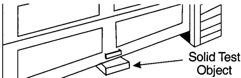
When the door reverses, remove the test object and run the full cycle of open and close of the door. Door should not reverse when it comes to the fully closed position.
