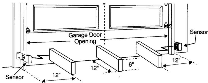
If the door does not respond properly to these tests, the Infrared Safety Sensors must be adjusted (refer to step 22 or 23 depending on type of sensors used). Repeat this test procedure. If the door opener still will not respond properly and fails this test, the door may cause severe injury or death. Have a qualified service person make repairs.
