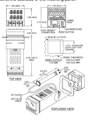
**Disassembly Instruction:** If necessary, the unit may be removed from the panel and opened.
