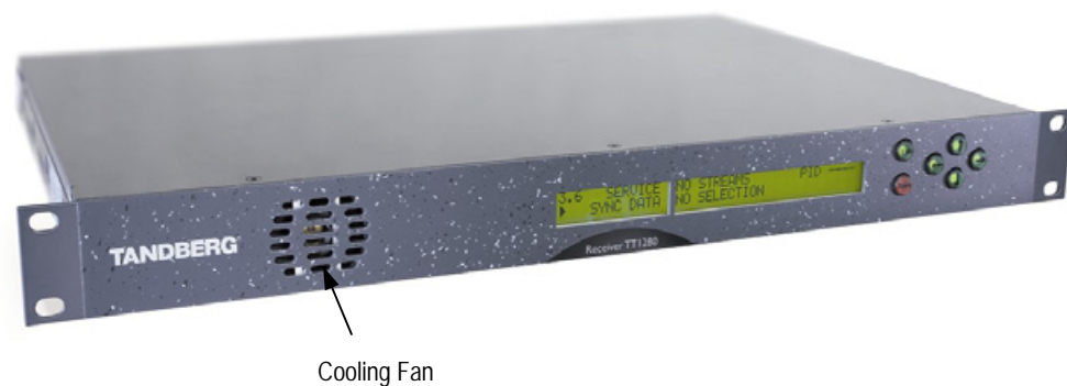
Figure 7.1: Cooling Fan Location
