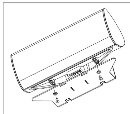
The wall-bracket cannot be pivoted from side to side. The bracket is not either designed to tilt up or down, and attempting to tilt it will damage the bracket and possibly the wall, which would not be covered by your warranty.
