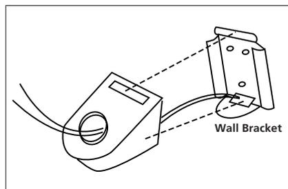
Insert the supplied bracket bolt up through the bottom of the bracket and terminal cover, and screw it into the threaded insert on the underside of the speaker. The bolt should be snug, but not so tight as to prevent the bracket from pivoting.
