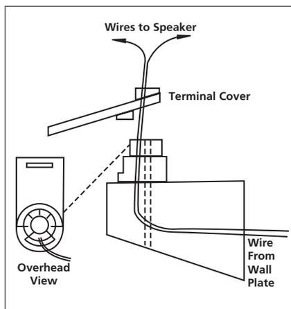
The bracket has two openings on top: a round screw hole, and an arc-shaped opening in front of it. The speaker cable should be threaded through the arc-shaped opening, not the screw hole.
