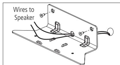
Position the bracket in such a way that the large hole for the cable is in front of the hole in the wall that holds the cable. Thread the cable through the hole and fix the bracket on the wall.
