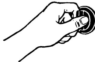
2. Line up openings in the reflector bowl with the surface unit receptacle and the element hold-down clip.
