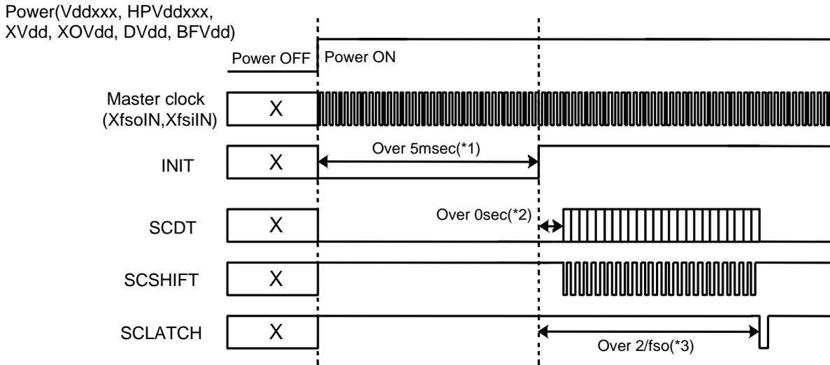
\*1 After a power supply and Master clock become to stable, INIT pin must be "L" over 5msec.
