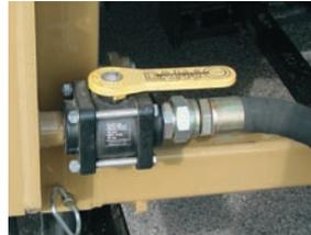
Shut-off valve permits maintenance without oil loss.
