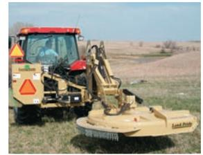
Hydraulic breakaway feature pivots arm backward to avoid obstacles and protect cutter arm. Hydraulically pivots back into place.
