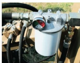
In-line filter cleans hydraulic fluid before it re-enters reservoir.
