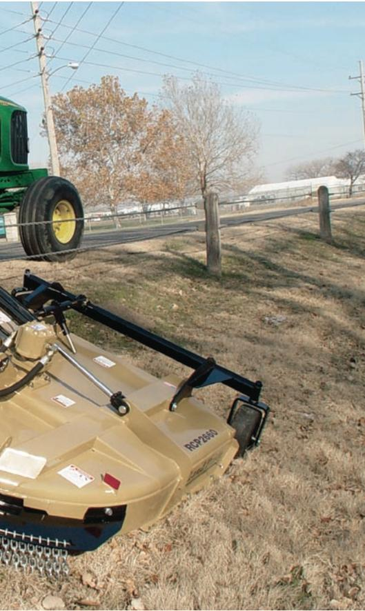
Optional gauge wheel deck allows the cutter to float over undulations without having to constantly monitor terrain conditions.
