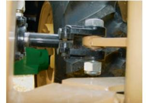
Cylinder shear-bolt breakaway for frame protection.
