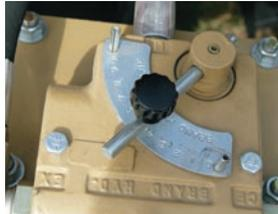
Flow control valve compensates for various hydraulic systems.
