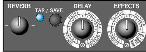
The Effects control selects the “pitch modified” and wah effects. Many of these effects have their speed controlled by the Tap/Save button. All of these effects have their speed controlled by the Tap/Save button. Additional information is provided on pages 5 and 10.
