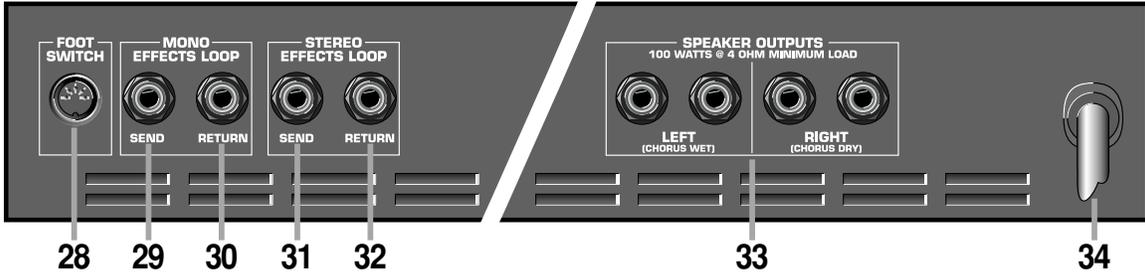
**28: FOOTSWITCH:** Use this jack to connect the footswitch cable (5-conductor midi cable) to the four-button footswitch (supplied). This allows you to remotely switch between the channels, set tap tempos, save new presets, and access a second set of DSP presets. (See page 9 for additional information.)
