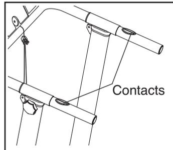
To measure your heart rate, **stand on the foot rails** and hold the metal contacts on the handrail. **Avoid moving your hands.** When your pulse is detected, your heart rate will be shown. **For the most accurate heart rate reading, continue to hold the contacts for about 15 seconds.**
