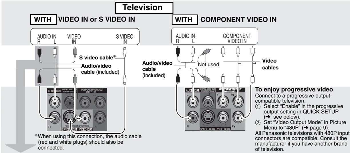
You can connect the audio cable to the 2-channel audio input terminals of an analog amplifier or system component to enjoy stereo.
