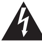
The lightning flash with arrowhead symbol, within an equilateral triangle, is intended to alert the user to the presence of uninsulated "dangerous voltage" within the product's enclosure that may be of sufficient magnitude to constitute a risk of electric shock to persons.
