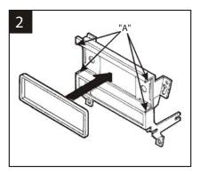
Locate the faceplate supplied with the aftermarket head unit. Place the faceplate into the recessed opening in the Radio Housing. If the faceplate fits easily into the opening with no interference, leave the Housing intact. If the faceplate does NOT fit easily into the opening, trim away the ribs located on the top and bottom of the opening ("A").
