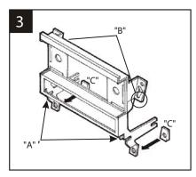
Convert the Radio Housing by cutting and removing the pins located under the equalizer opening ("A"). Trim no less than 1/8" and no more than 1/4" from the bottom of each upper mounting tab ("B"). Snap the Prizm Spacers onto the back of the lower mounting tabs ("C").
