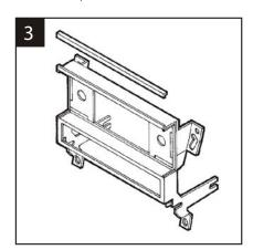
Locate the v-cut along the top lip of the Radio Housing. Using the v-cut as a guide, cut and remove the top portion of the Housing as indicated above.
