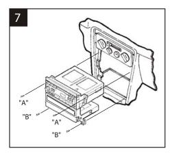
COROLLA: Re-connect the battery terminal and test the unit for proper operation. Mount the head unit/kit assembly to the sub-dash with (4) Phillips screws previously removed in step #1.
