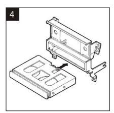
Remove the cupholder from the factory head unit assembly. Slide the cupholder into the bottom of the Radio Housing until the locating pins engage the slots in the kit. (Once the locating pins are engaged, maneuver the cupholder until it is flush with the face of the Housing). Skip to the Installation Instruction for ALL VEHICLES on Page #3.
