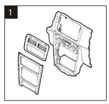
Disconnect the negative battery terminal to prevent an accidental short circuit. Unclip the radio trim bezel (upper dash). Remove (4) Phillips screws from the factory head unit, slide the unit out and disconnect the wiring. Remove the ashtray and unclip the trim bezel (lower dash). Remove (4) Phillips screws from the factory pocket/cupholder assembly and remove the assembly. (Metra recommends ordering the 88-00-8000 or 88-00-9000 to fill the space left in the upper dash location).
