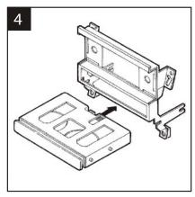
Remove the cupholder from the factory head unit assembly. Slide the cupholder into the bottom of the Radio Housing until the locating pins engage the slots in the kit. (Once the locating pins are engaged, PUSH the cupholder into the Housing until it stops). Skip to the Installation Instruction for ALL VEHICLES on Page #3.
