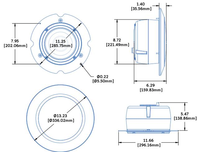
The Stella-8C ceiling mount installation loudspeaker is a self-powered loudspeaker engineered primarily for use in Meyer Sound’s Constellation electroacoustic architecture. Housed in an aluminum die cast enclosure with a heatsink on the back, the Stella-8C can be flush-mounted in ceilings and walls with standard backboxes for 8-inch drivers (with a minimum depth of 6.5 inches).
