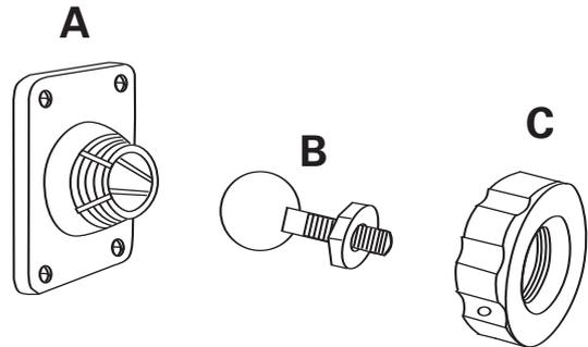
**Step 4.** Screw the ball and shaft assembly (B) to the lower 1/4"-20 insert on the rear of the satellite. Back out 1/2 of a turn and tighten the nut against the speaker.
