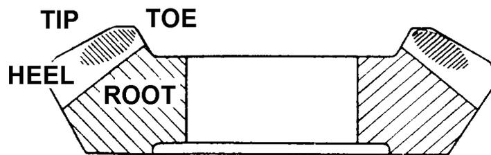
Contact markings closer to toe and root than factory markings.
