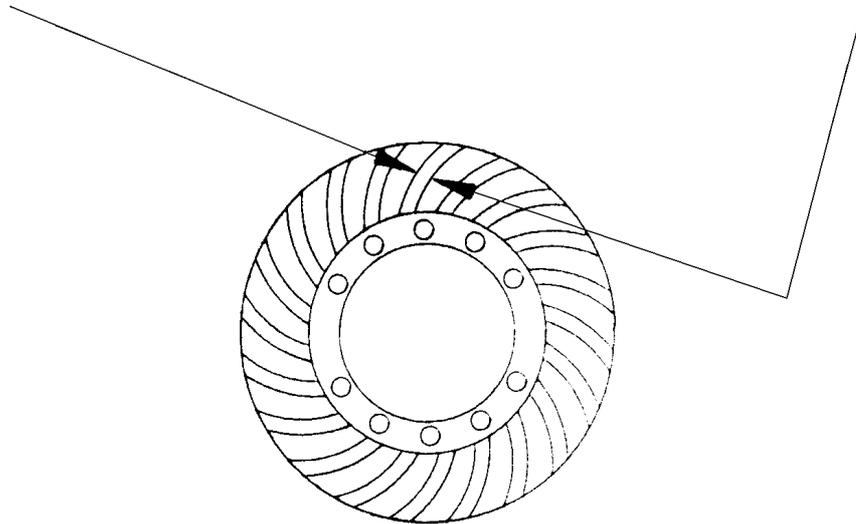
The markings on a crownwheel which is correctly meshed with the pinion should resemble those shown on the illustration below:-
