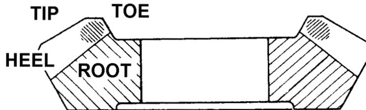
Contact markings closer to toe and tip than factory markings
