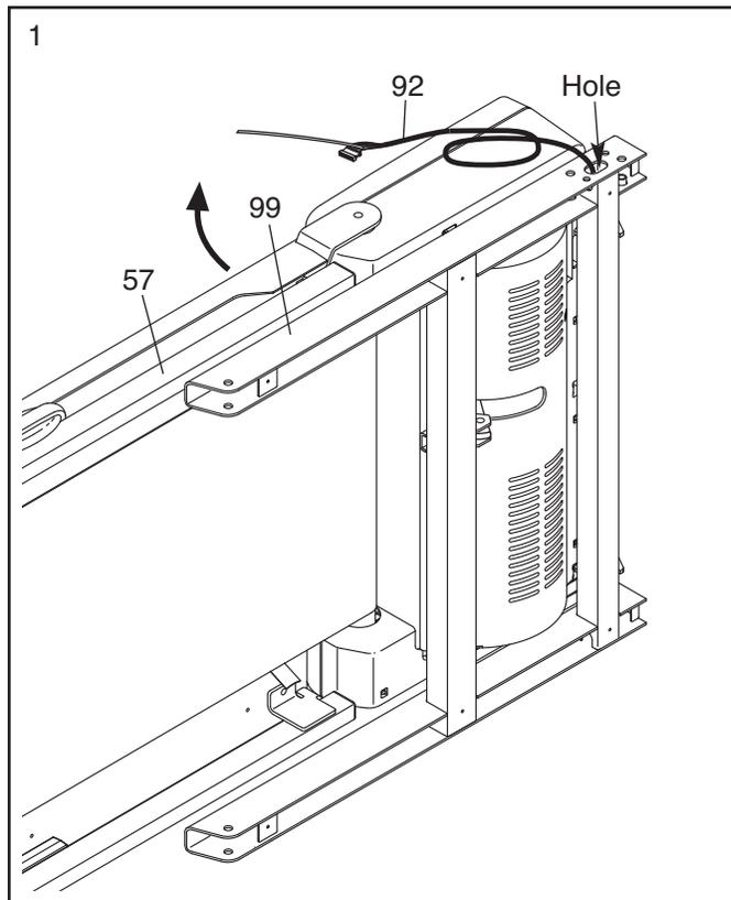
2. **See the inset drawing.** Cut the plastic tie near the Wire Harness (92).
