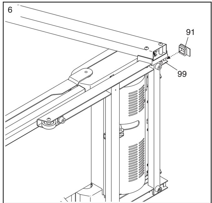
7. With the help of a second person, carefully tip the treadmill onto its right side. Partially fold the Frame (57) so that the treadmill is more stable; **do not fully fold the Frame yet.**
