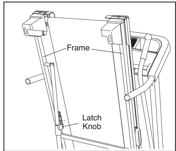
2. Hold the metal frame firmly with both hands and lower it to the floor. **CAUTION: Do not grip only the plastic foot rails or drop the frame to the floor. Bend your legs and keep your back straight.**
