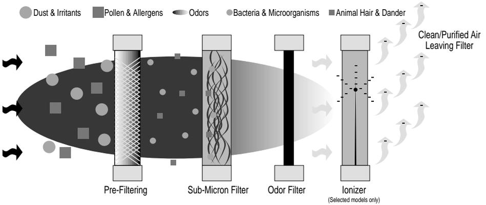
The above is an illustration of how the *HEPAtech*<sup>TM</sup> air purification systems work. Dust and other irritants are pulled into the air purification system and cleaned through the *HEPAtech*<sup>TM</sup> Filter. Clean, purified air is released into the room.
