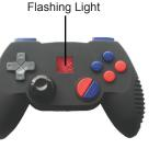
Battery Indicator: A red light will flash when the buttons are pressed indicating the batteries are ok.
