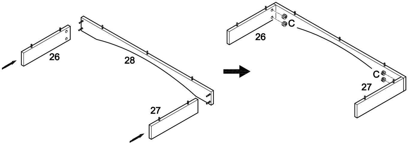
Attach slats (26,27) to slat (28) using cam bolts as guides. Insert cam locks (C) into slats (26,27) and tighten with a screwdriver.
