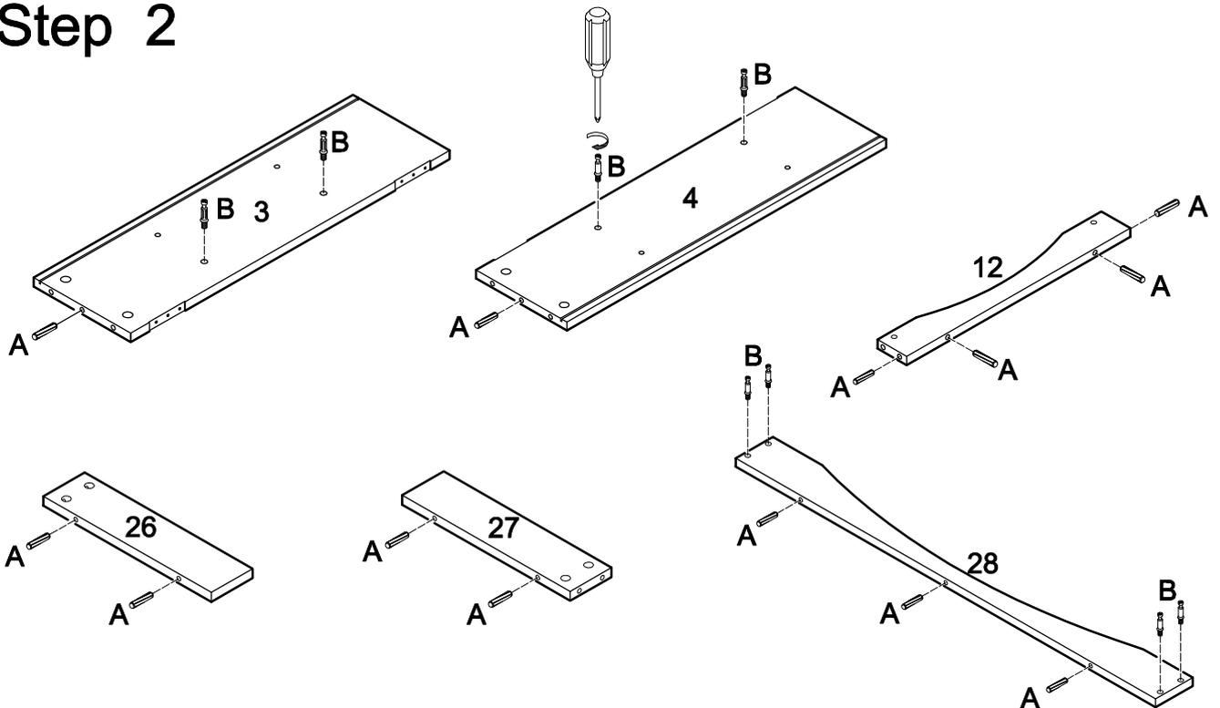
Screw cam bolts (B) into panels (3,4) and slat (28). Insert dowels (A) into panels (3,4) and slats (12, 26,27,28).
