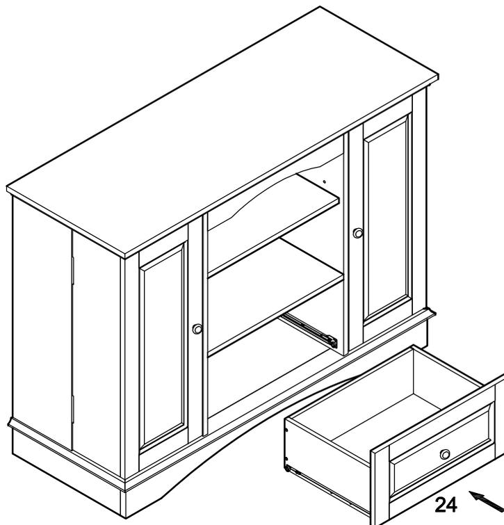
Carefully slide the drawer into the stand assembly.
