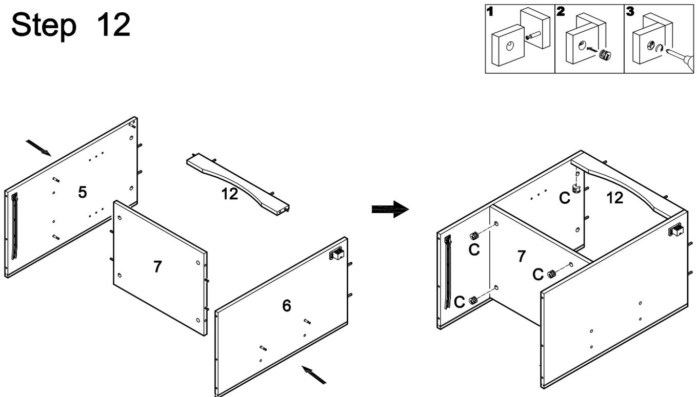
Attach panels (5,6) to panel (7) and slat (12) using cam bolts and dowels as guides. Insert cam locks (C) into panel (7) and slat (12) and tighten with a screwdriver. *Note that four cam locks will be inserted into panel (7), and two will be inserted into slat (12).*
