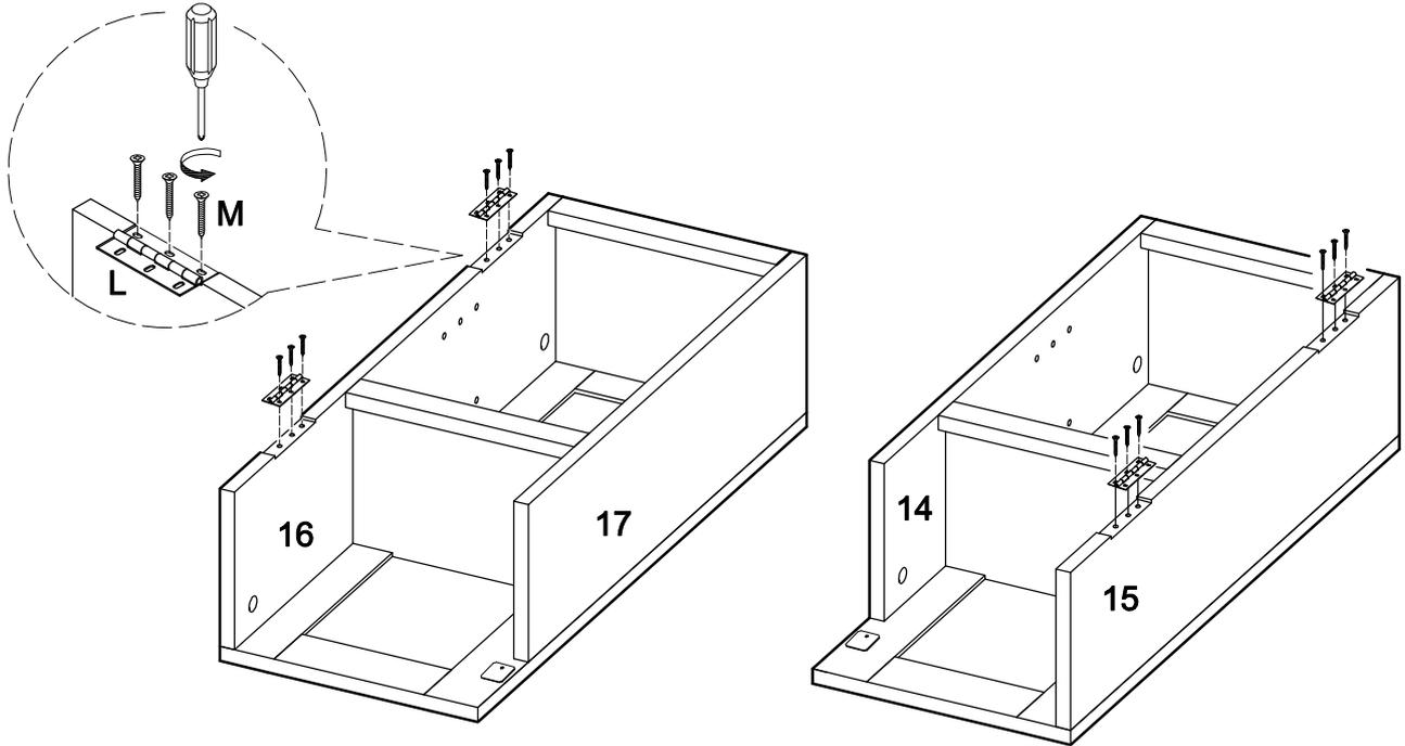
Attach hinges (L) to panels (15,16) using large screws (M).
