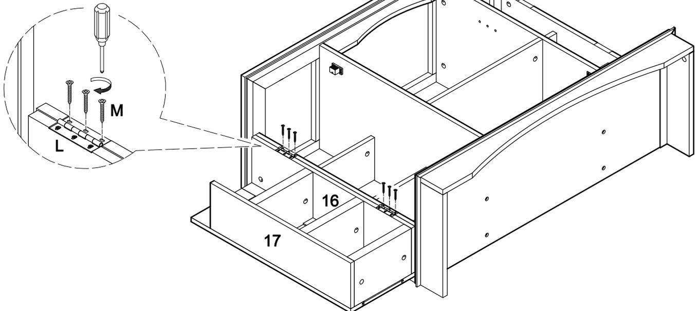
Attach the door (16,17) assembly to the stand assembly at hinges (L) using large screws (M).
