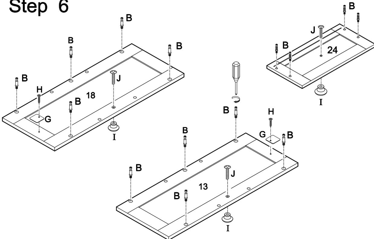
Screw cam bolts (B) into doors (13,18) and drawer front (24). Attach handles (I) to doors (13,18) and drawer front (24) using small bolts (J). Attach door stopper plates (G) to doors (13,18) using small screws (H).
