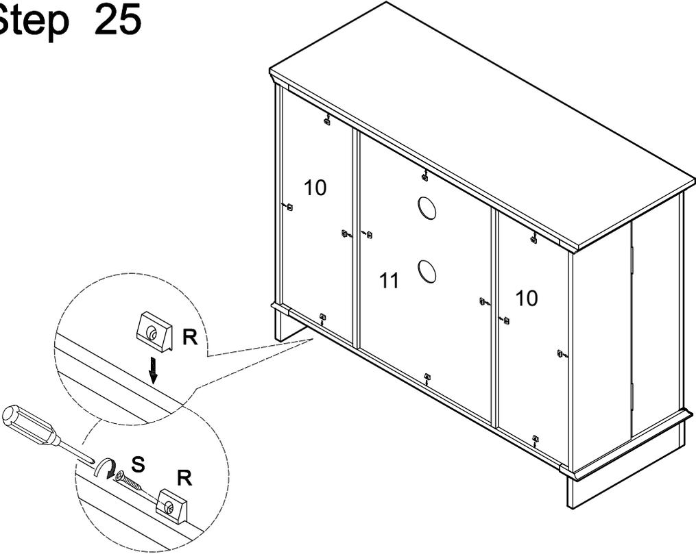
Secure back panels (10,11) using plastic wedges (R) and medium screws (S).
