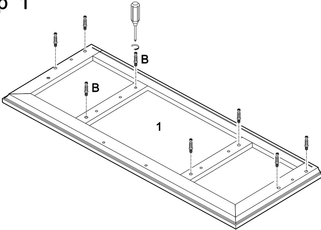
Screw cam bolts (B) into top panel (1).
