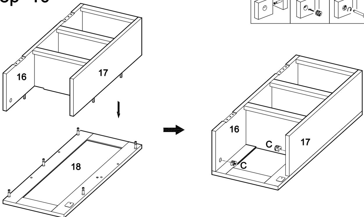
Attach the shelf assembly from Step 8 to door (18) using cam bolts and dowels as guides. Insert cam locks (C) into panels (16,17) and tighten with a screwdriver. *Note that three cam locks will be inserted into panel (16) and two will be inserted into panel (17).*
