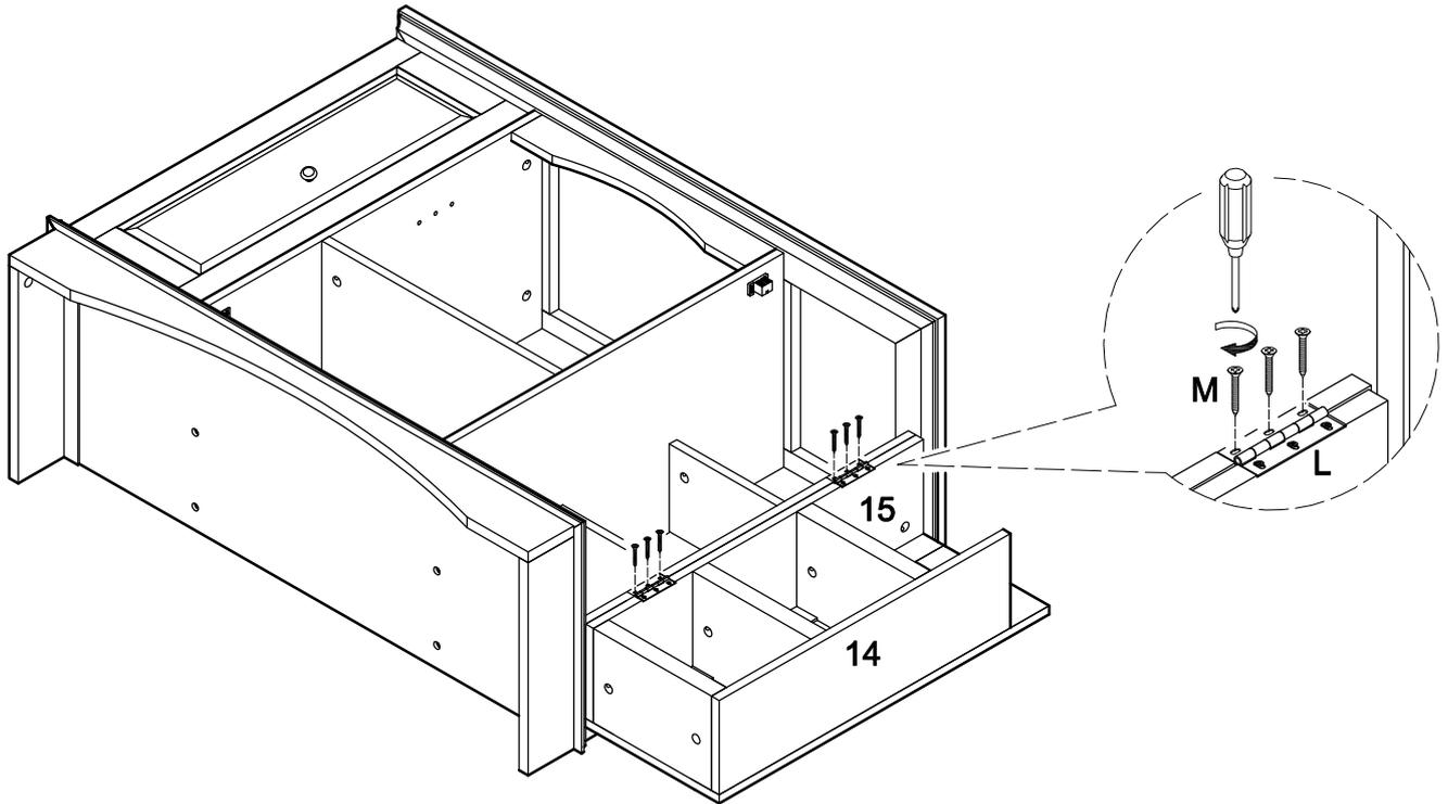
Attach the door (14,15) assembly to the stand assembly at hinges (L) using large screws (M).
