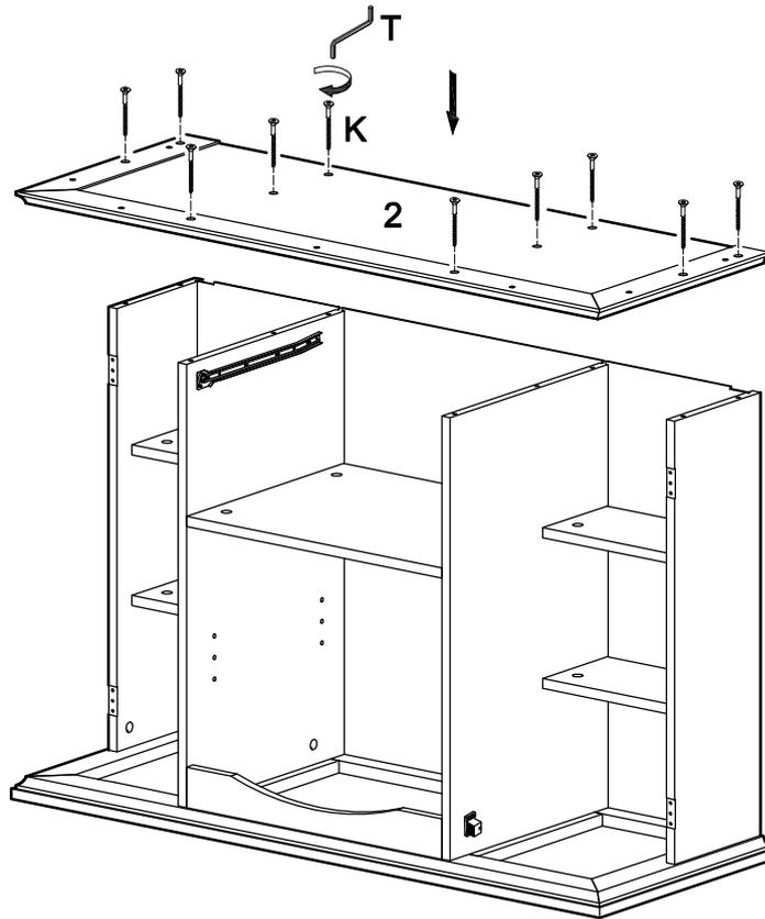
Attach bottom panel (2) to the frame assembly using large bolts (K) and wrench (T).
