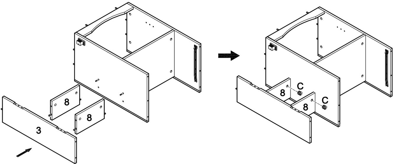
Attach shelves (8) to the frame assembly from Step 12, then attach panel (3) to shelves (8) using cam bolts and dowels as guides. Insert cam locks (C) into shelves (8) and tighten with a screwdriver. *Note that two cam locks will be inserted into each shelf.*
