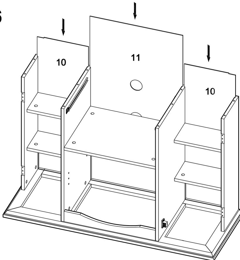
Slide back panels (10,11) into the frame assembly. Note that the back panels will slide down in the grooves along the back of the frame assembly.
