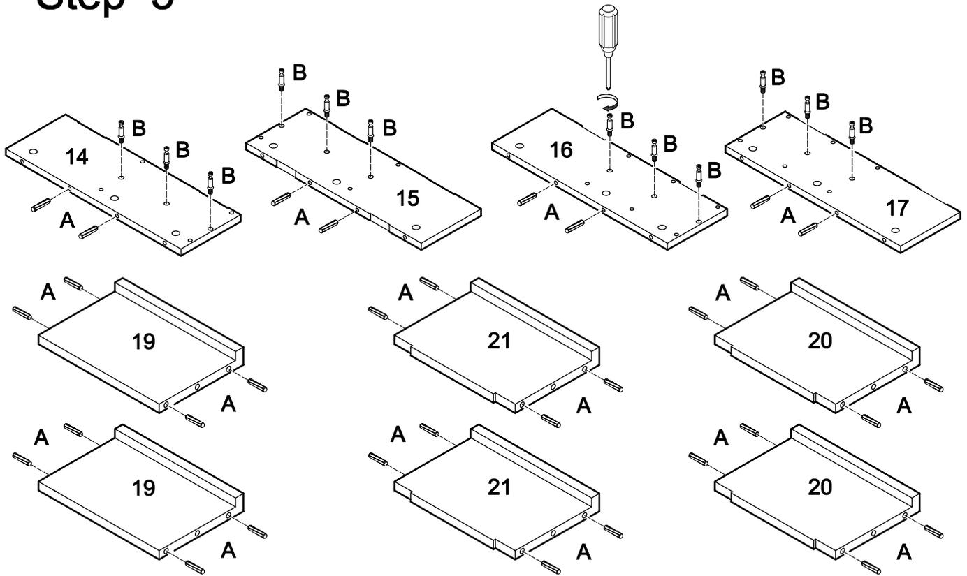
Screw cam bolts (B) and insert dowels (A) into panels (14,15,16,17). Insert dowels (A) into shelves (19,20,21).
