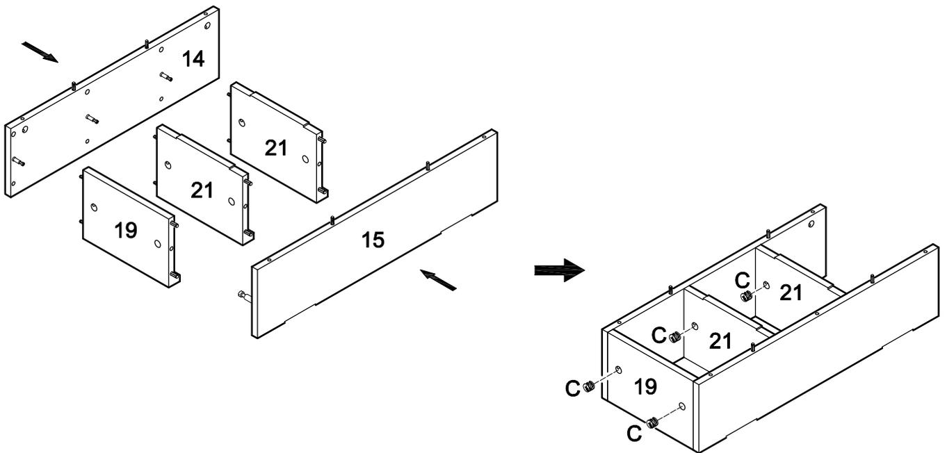
Attach shelves (19,21) to panels (14,15) using cam bolts and dowels as guides. Insert cam locks (C) into shelves (19,21) and tighten with a screwdriver. *Note that two cam locks will be inserted into each shelf.*
