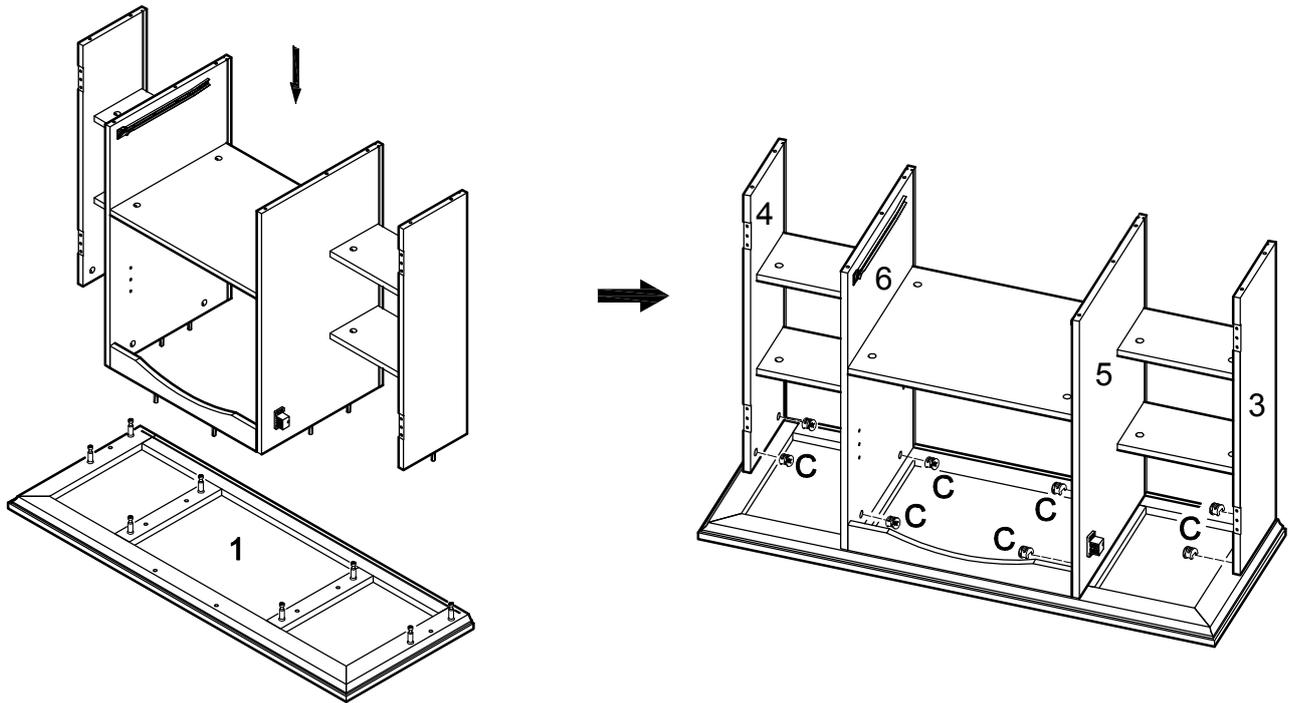
Attach the frame assembly from Step 14 to top panel (1) using cam bolts and dowels as guides. Insert cam locks (C) into panels (3,4,5,6) and tighten with a screwdriver.
