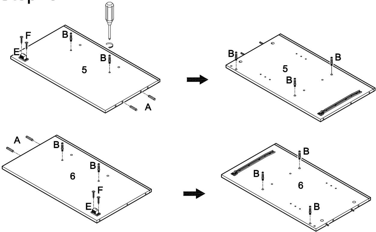
Screw cam bolts (B) and insert dowels (A) into panels (5,6). Attach door stoppers (E) to panels (5,6) using round-head screw (F). Flip panels (5,6) over and screw in cam bolts (B).
