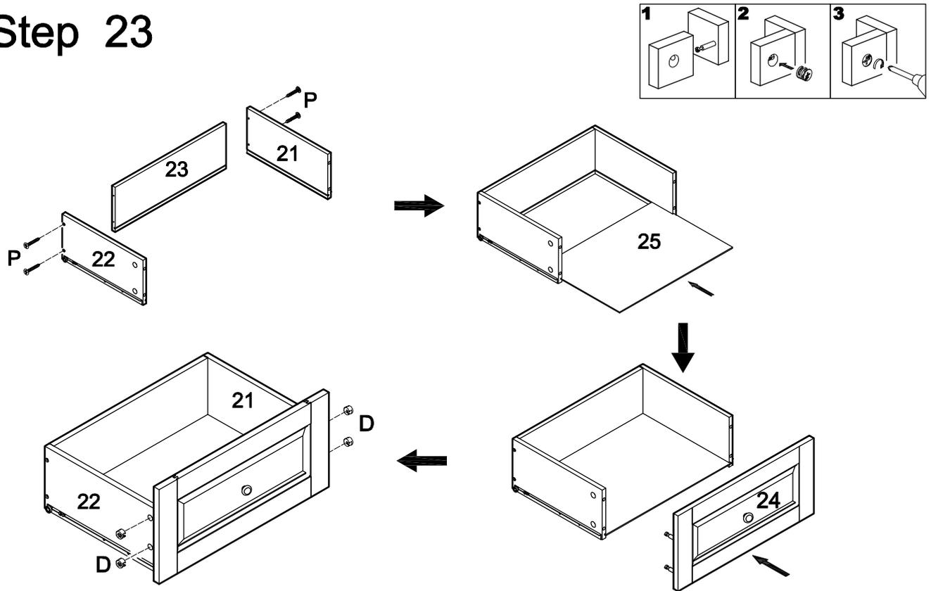
Attach drawer sides (21,22) to drawer back (23) using extra-large screws (P). Slide drawer bottom (25) into the drawer assembly. Attach drawer front (24) to the drawer assembly using cam bolts as guides. Insert small cam locks (D) into drawer sides (21,22) and tighten with a screwdriver.
