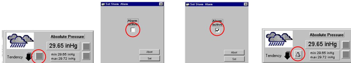
**Note:** The alarm bell icon may not appear immediately on the Heavy Weather program since it may take few seconds for the program to calculate and confirm the setting
